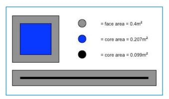
Taking a flow rate of 0.5m<sup>3</sup>/s and the coefficient, based on core area, of 0.44, the pressure loss would be:
